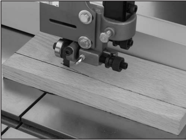
Figure 29. Blade leading away from line of cut.
